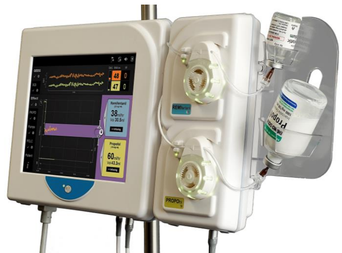
Fig. 12 – AutoTIVA (model AT-901) closed-loop TIVA delivery system. Advanced prototype product and research platform (not for sale).
